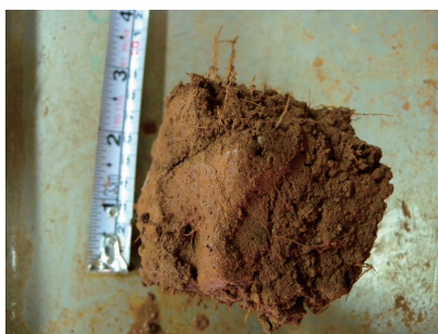
圖 7 拉拔試驗用之百喜草含根土塊 Fig.7 Bahia grass rooted soil block for pull-out test
