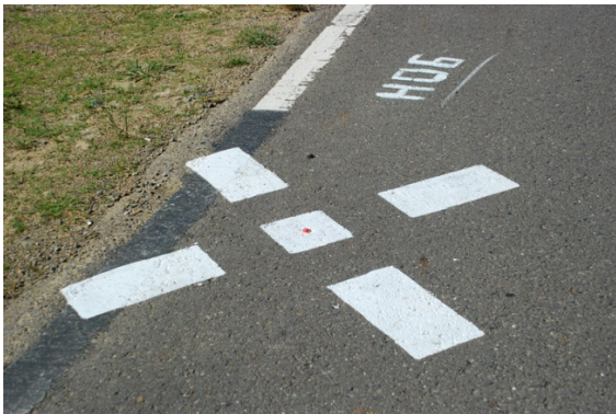
Fig.7(a) Common ground control point for aerial photogrammetry in Taiwan
