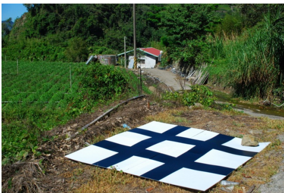
Fig.7(b) Self-developed ground control point
