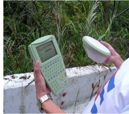
Fig.6(a) VBS-RTK receiver and antenna (Model No.: Leica ATX1230 GG)
